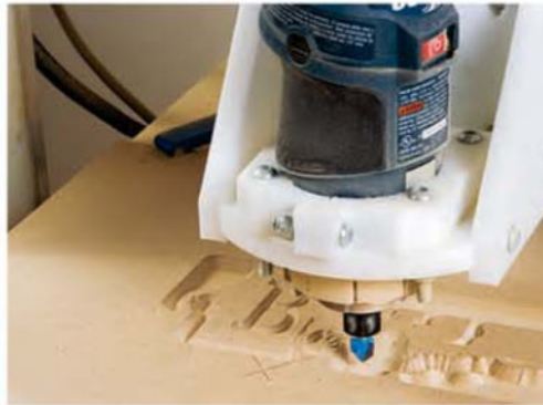
The software directs the CNC Shark's router-powered cutter. The Shark performs much more like a full-sized standard CNC router.
