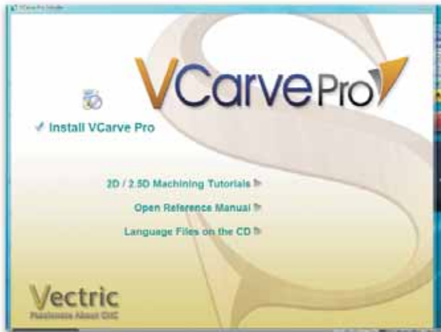
Photo.4: VCarve provides tools to create, manipulate and view designs, calculate toolpaths, estimate cutting times, and generate code to drive the CNC Shark
