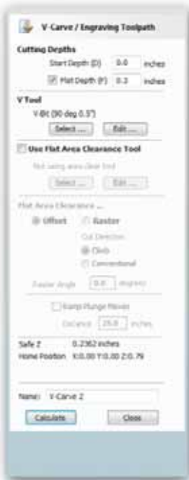
Photo.10: When the design has been completed, the tool and the cutting parameters selected, the toolpath and estimated time can be calculated
